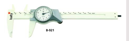
These low cost calipers are made from glass fibre reinforced superpolyamid. Light weight and easy to handle, with a clearly marked dial helps reduce reading errors.
